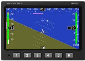
User interaction takes place via the EFIS-D60 main display and the six buttons beneath.
