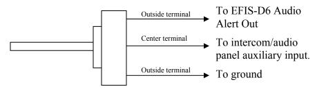
To set the volume of the AOA alarm, you will need your EFIS-D6 powered on and the alarm output wired as described above. Enter the EFIS menu by pressing any button (except the leftmost or rightmost) beneath an EFIS page. Press SETUP > AOAALM. In that menu, press the TEST button. While the button is held down, the AOA alarm will sound. Adjust the variable resistor until the volume in the intercom or audio panel is at an acceptable level.
