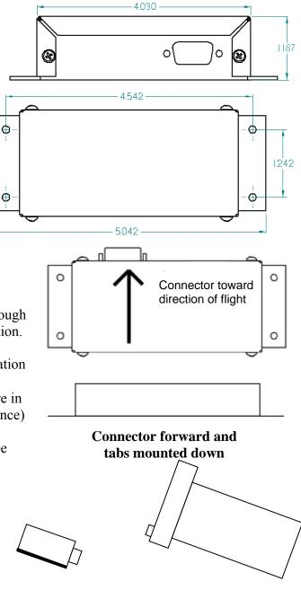
Side view of EDC-D10A, tabs mounted down and aligned within 1 degree of pitch with EFIS-D6 D10A is aligned with the EFIS-D6 to better than 1 degree.
