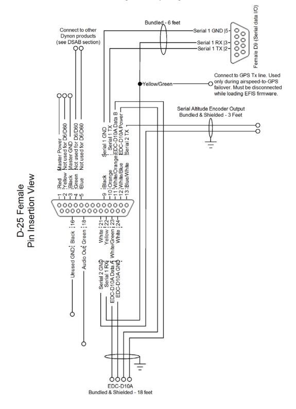
The pin assignments for the female 25-pin harness are repeated below. *Note that the pin numbers are labeled on the face of both the female and male connector*. Each connection on the harness supplied by Dynon is color-coded. These colors are listed in the following chart.
