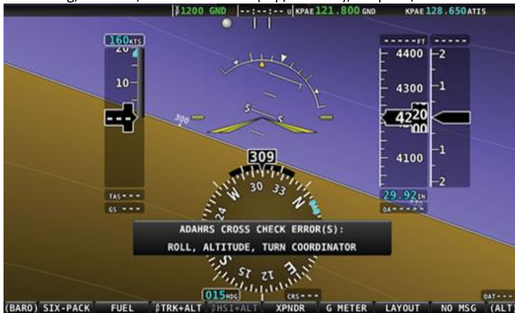
Figure 26 – ADAHRS Cross-Checking Disagreement
