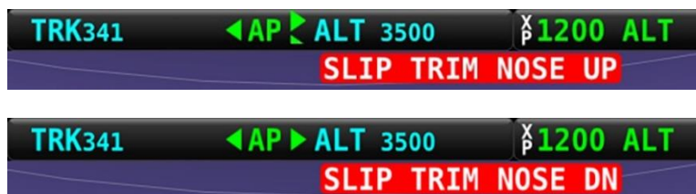
Figure 47 – Pitch Slip Trim Nose Up / Down Alerts
