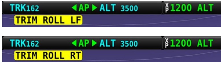
Figure 48 – Roll Trim Left and Right Alerts
