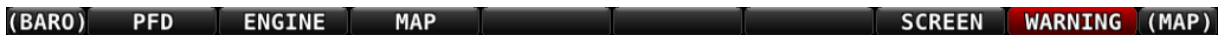
Figure 107 - Message Notification Area above button 8 (2nd from right), showing a Warning Notification
